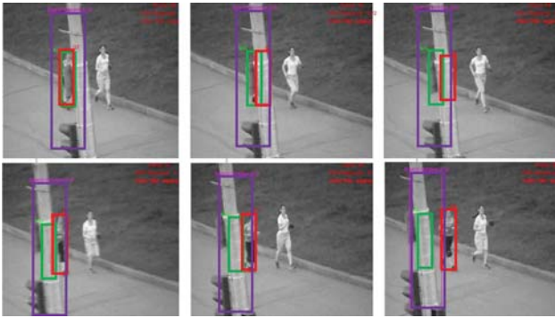
Fig. 9. In jogging video, a Kalman filter is not used. Ground Truth positions (red) and HOG estimates (green) are each represented by a bounding box. Track is lost due to occlusion. Once the object leaves the detection window (purple), track cannot be easily reestablished.
