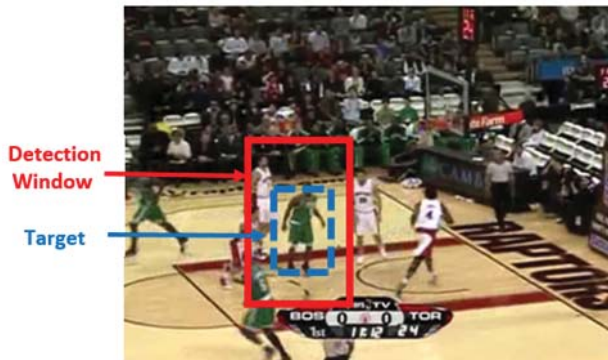
Fig. 5. Image shows Detection Window "Patch (red box)". Target object shown in (blue box). HOG scan conducted in Detection Window only to facilitate real-time tracking.
