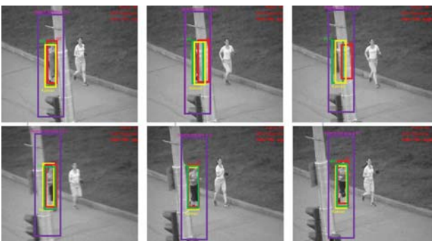
Fig. 10. In this frame sequence, a Kalman filter (yellow bounding box) is used. Both HOG estimates and Ground Truth positions are also shown with bounding boxes. Track is maintained during occlusion event.
